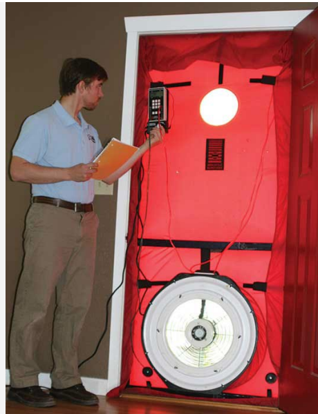
Efficiency experts use a blower-door test to determine how drafty a house is, measured in air changes per hour (ACH).
